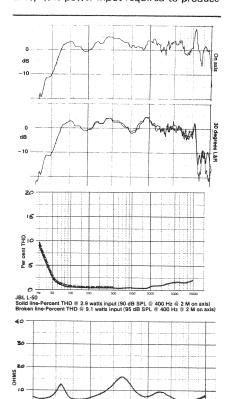
90 dB SPL at 400 Hz at 6 feet on axis) was 2.9 watts. The system resonance frequency was found to be 61 Hz.
